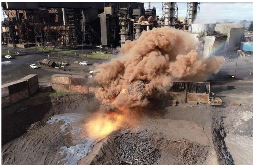
Figure 8.3: Fume generated during an unsuppressed iron plating event
