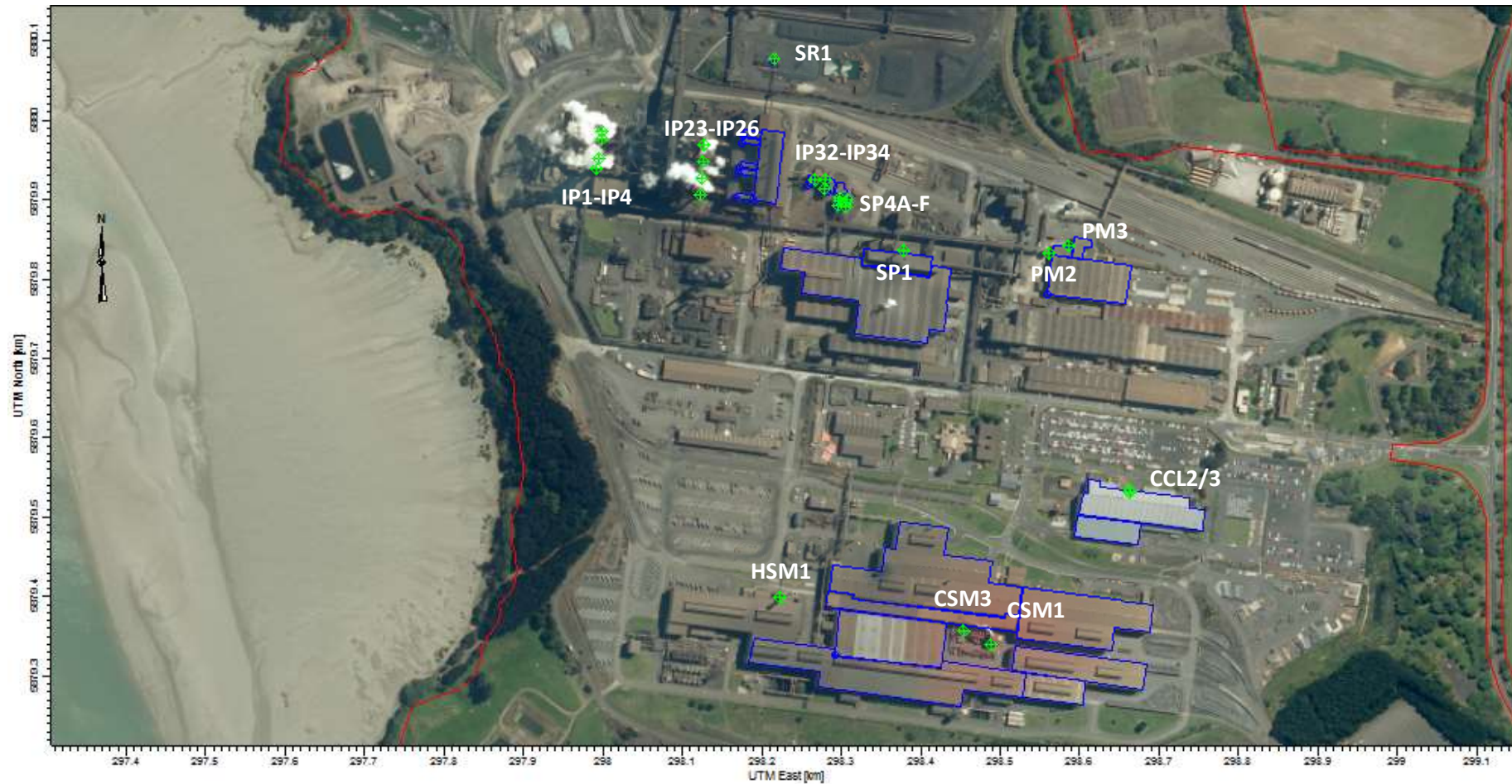
Figure 3.1: Main stack emission sources (green crosses). Note: the blue shapes indicate the buildings included in the model for the purpose of evaluating building downwash effects
